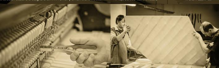
Gluing the soundboard onto the backframe.
